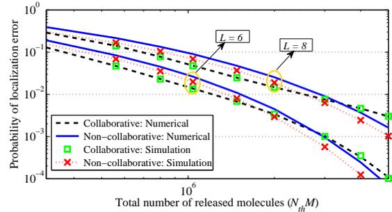
Fig. 3. The probability of error vs. total number of released molecules [8].
